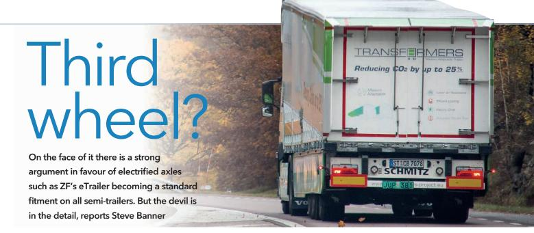
he axle's intelligent electric motor recuperates energy which would otherwise be lost during braking or when the truck coasts downhill.
